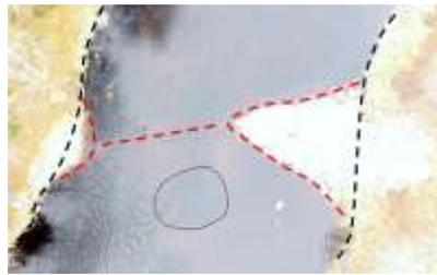
*An overhead view of a rock sill and deflector on the main branch, West River. This section of river is 2-3 times as wide as it should be, largely as a result of historical log driving. These deflectors help to establish a deeper channel, while the sill causes the water to dig pool habitat (circled area). The increased flow reduces ice formation in winter and keeps the stream temperature relatively cooler in summer.*
