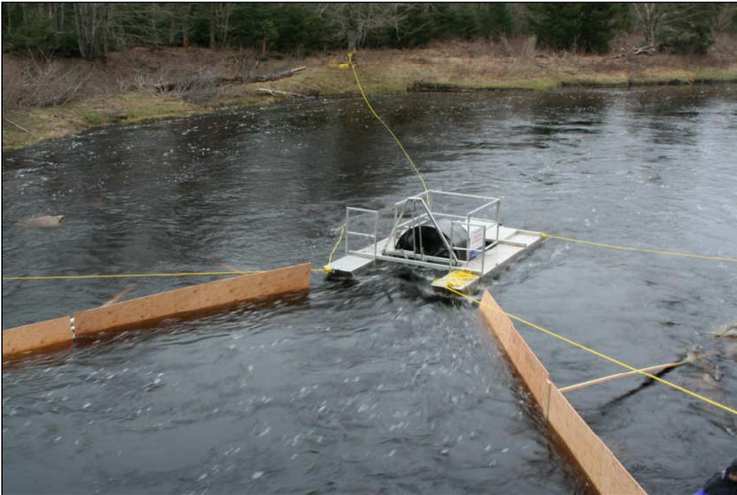
Figure 7 - Smolt wheel in operation prior to the flood of late April / early May.
